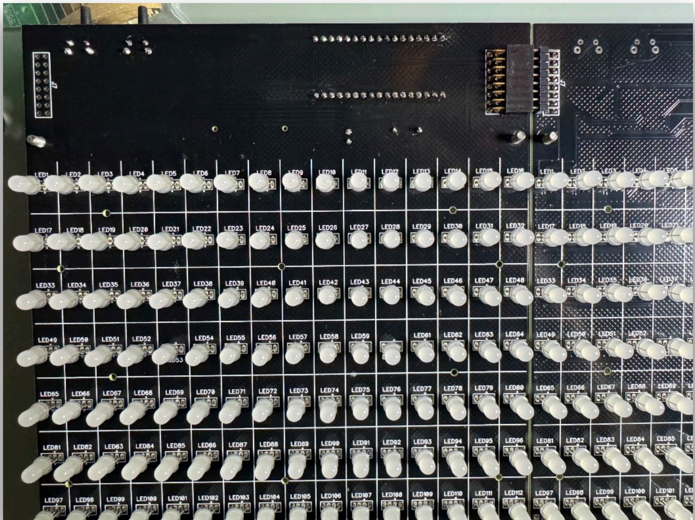
For a multi-board clock, note the installation of the right angled connectors, the left hand board is the processor board and the right hand the add-on display
