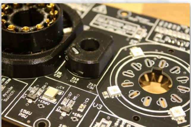
This completes the assembly of the display board (except for inserting your lovely E1T tubes that is, followed by the light guides).<sup>32</sup>
