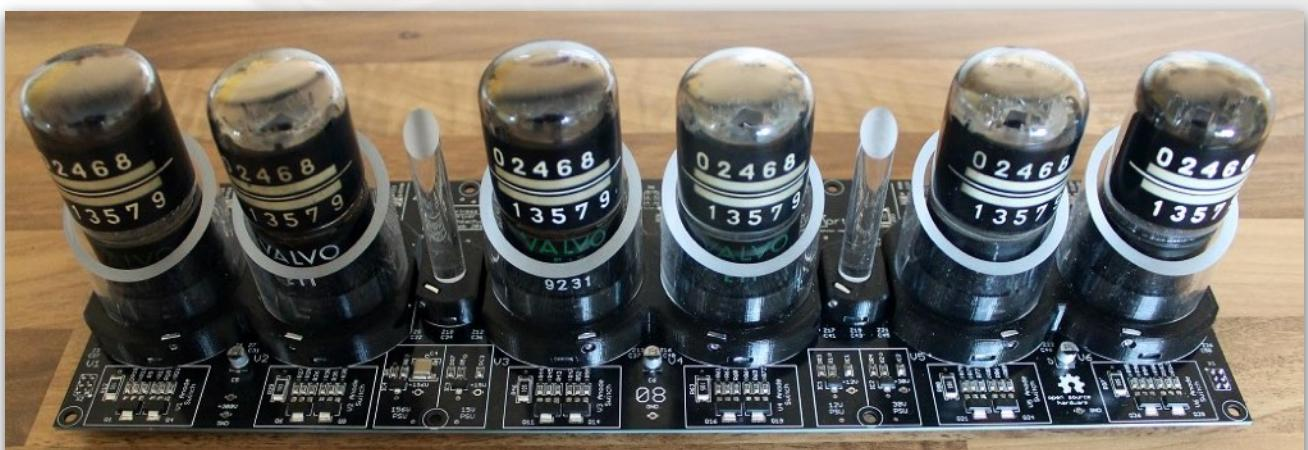
Completed Display Board With Light Guides and E1T's
