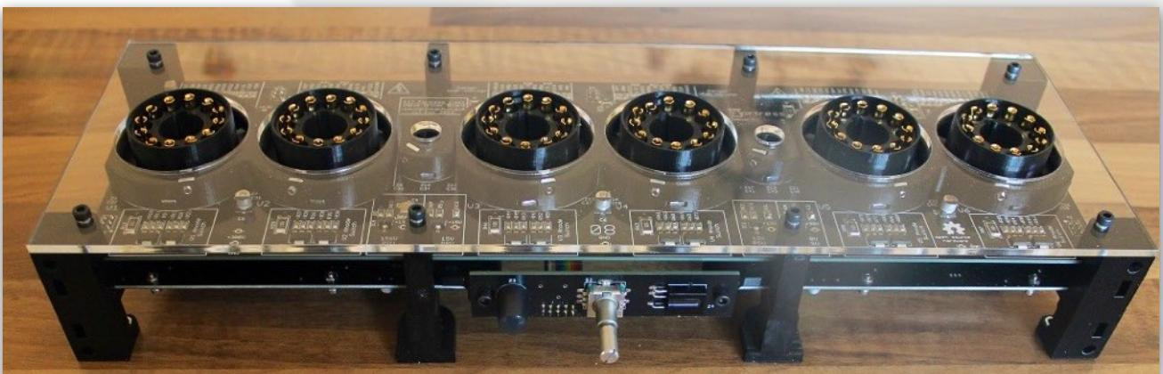
From Step 7 - Top acrylic attached to 3D printed posts
