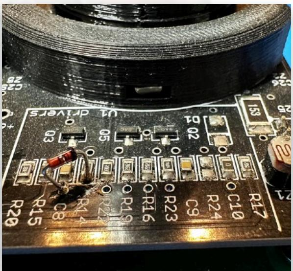
V1 Driver Station Diode Installation
