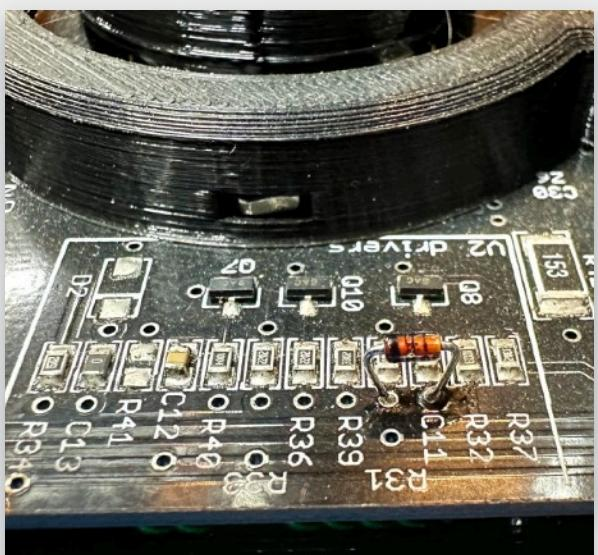
V2 Driver Station Diode Installation
