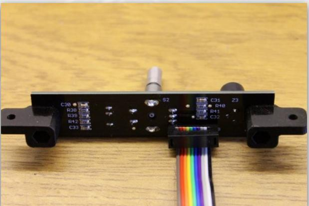
**Rear View of Control Sub Board with 3D Mounts**
