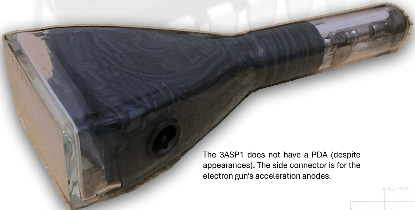
A 3ASP1 CRT as an example of a rectangular display with a high X/Y ratio
