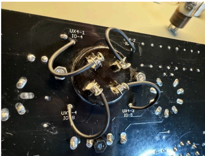
Wiring up the UX4 socket to the PCB
