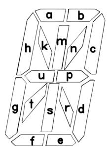
Segments will be off if 0 is in that segment's position, and on with 1. Comments can be entered after the 16<sup>th</sup> character on each row. Any text editor that does not add control characters can be used to edit the file, including Notepad on Windows. Notepad++ is a free text editor that offers many additional features. Below is an example from the English font file on the SD card. Its path is /English/English.fnt.
