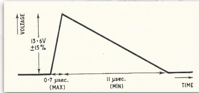
Fig 5.9 - An Input Pulse Suitable for the Operation of the E1T
