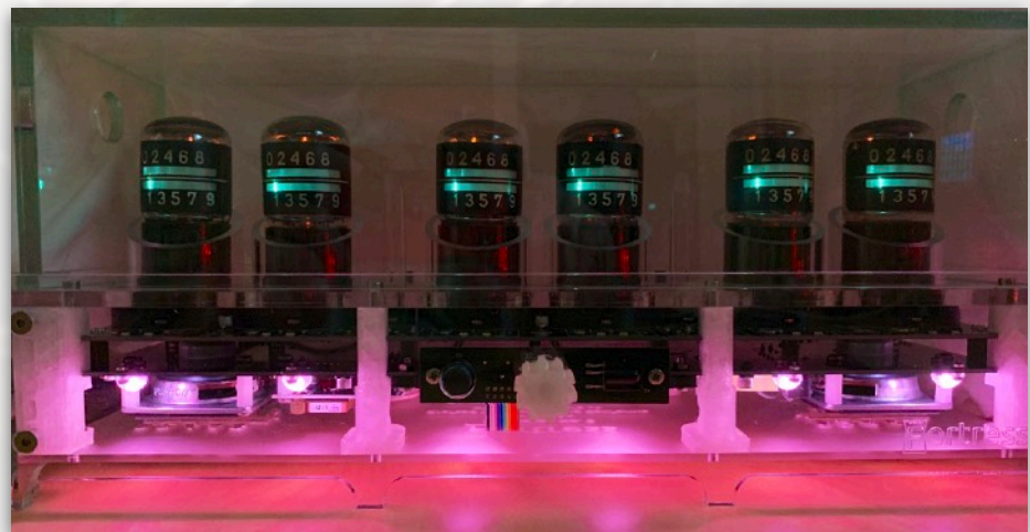
Powering up the Fortress - E1T tubes counting down on startup
