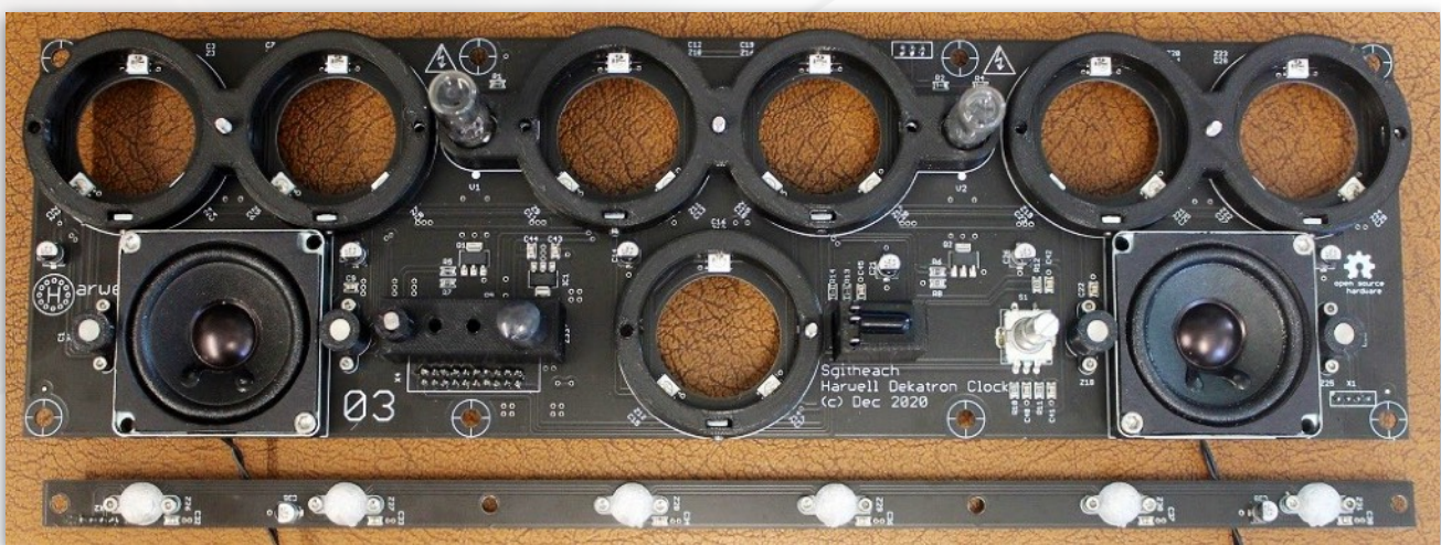
Component side - All through hole parts installed and 3D printed parts fitted
