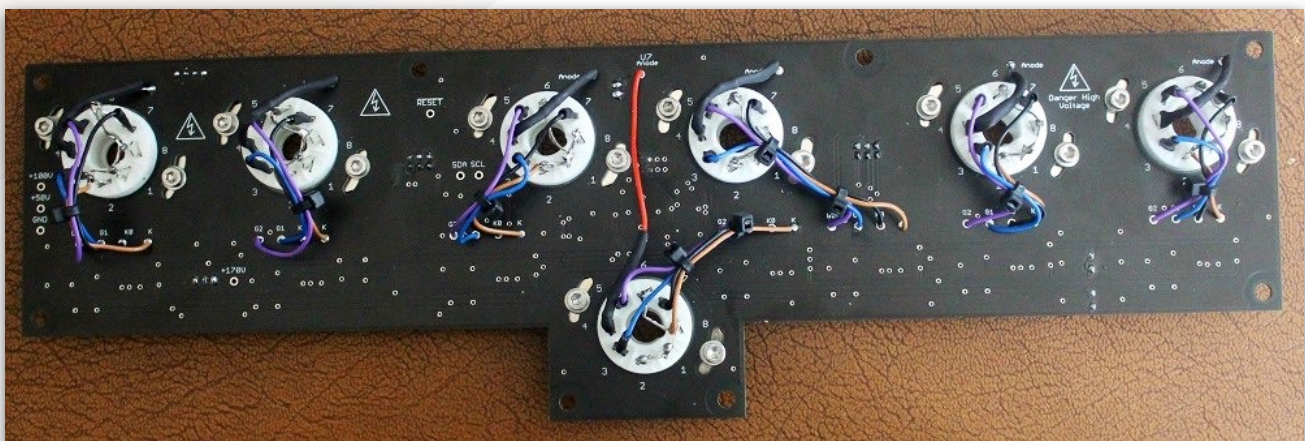
Dekatron Driver Board Completed - British GC10 and GC12/4B Dekatron
