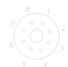
Base Connections (underside view)
