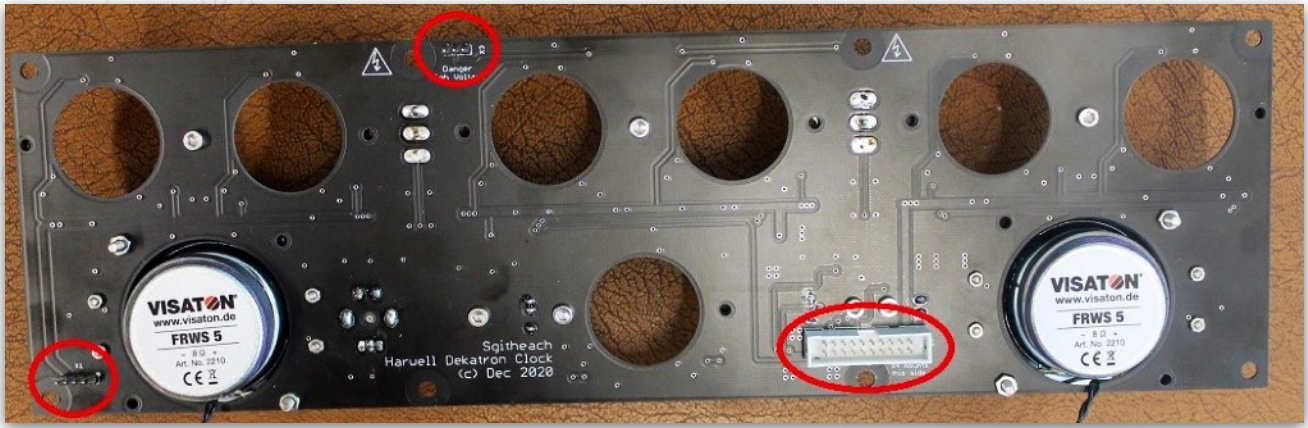
Rear (copper) side - Highlighted in red are X1, X3 and X4 fitted on this side
