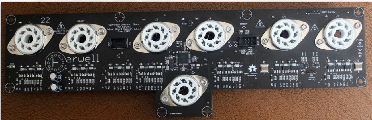
Dekatron Driver Board Completed - British GC10 and GC12/4B Dekatron
