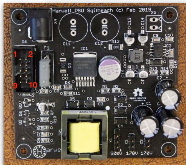
The Completed PSU Board (note numbers on X6 for orientation)
