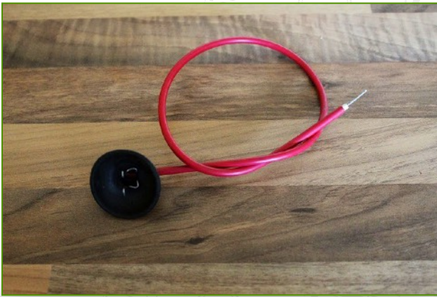
[Left]: A pukka PDA wire and cap - safety first! [Right]: An example of a PDA socket on a CRT
