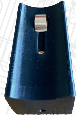
With the Be-Cu Finger Stock glued in place
