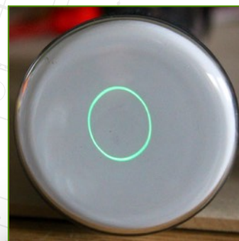
Photo 10: Sine and cosine waves applied to the X and Y deflection plate connections
