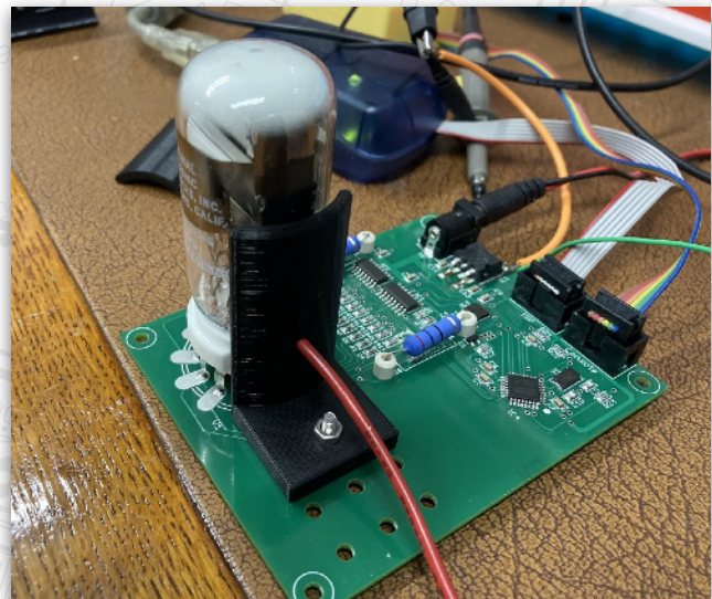
Mounted in place on the NIMO tester board
