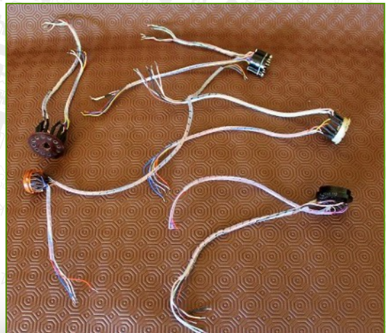
A range of CRT bases permanently wired for use with the CRT Tester. As I test CRTs I make up a permanent wired base if it is a type that I am likely to use again.
