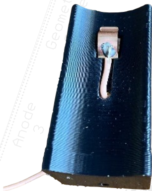
EHT (3kV rated) wire soldered and routed down the slot and through the hole
